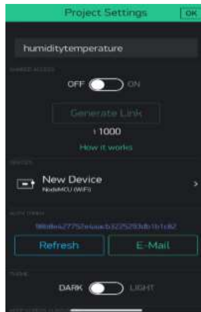
Figure 7: Create a new project at Blynk App
