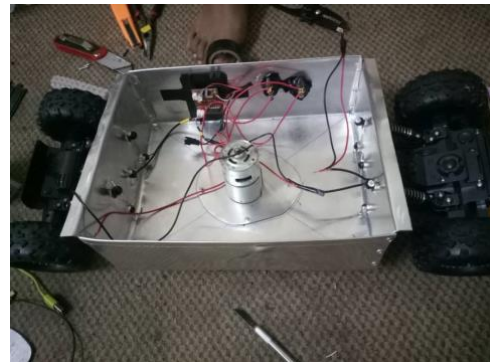
Figure 7: Installation of DC Motor and blade
